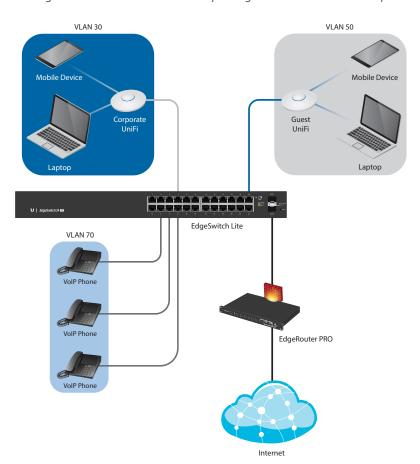
VLANs for Corporate Wireless, Guest Wireless, and VoIP For wireless access, two Ubiquiti UniFi®Access Points connect to the EdgeSwitch Lite.
