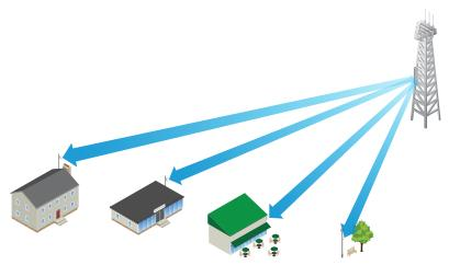
The NanoBeam ac used as a CPE device for each client in an airMAX PtMP network.
