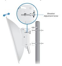
10. Lock the alignment by tightening the eight hex head bolts to 25 N-m.
