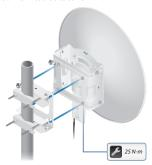
Before adjusting the azimuth and elevation angles, ensure that these eight hex head bolts are loose enough to allow movement.
