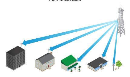
The PowerBeam 2AC used as a CPE device for each client in an airMAX PtMP network.
