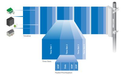
Up to 100 airMAX ac stations can be connected to an airMAX ac Sector; four airMAX ac stations are shown to illustrate the general concept.
