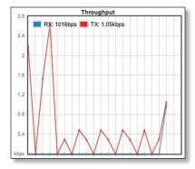
Throughput displays the current data traffic on the port in both graphical and numerical form. The chart scale and throughput dimension (bps, kbps, Mbps) change dynamically depending on the mean throughput value. The statistics are updated automatically.
