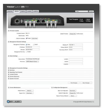
5. You can enable PoE on the *Ports* tab and customize additional settings as needed.
