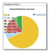
A pie chart, *Packet Distribution*, displays the current packet sizes going through the port. The pie chart is updated automatically.
