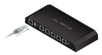
Connect Ethernet cables from the Ethernet ports of your devices to the numbered ports of the TOUGHSwitch.
