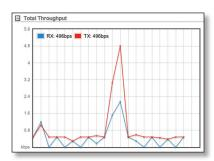
Total Throughput displays the current data traffic on the TOUGHSwitch in both graphical and numerical form. The chart scale and throughput dimension (bps, kbps, Mbps) change dynamically depending on the mean throughput value. The statistics are updated automatically.
