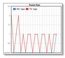
Packet Rate displays the current packets per second rate on the port in both graphical and numerical form. The chart scale and packet rate dimension change dynamically depending on the mean packet rate value. The statistics are updated automatically.
