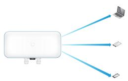
MU-MIMO with 2x2 and 1x1 clients: Each client radio of the UniFi WiFi BaseStation XG communicates with one 2x2 client and two 1x1 clients at a time.
