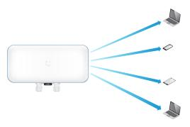
MU-MIMO with 1x1 clients: Each client radio of the UniFi WiFi BaseStation XG communicates with four 1x1 clients at a time.
