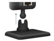
4. Attach the airCam Mini to the Wall Mount Bracket.
