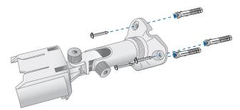
Note: There are three recessed areas for the Ethernet cable on the *Mounting Bracket Base*. Place the Ethernet cable in the recessed area that will be nearest to your power source.
