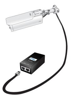
2. Connect an Ethernet cable from your LAN to the Ethernet port labeled **LAN** on the *PoE Adapter*.
