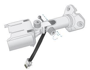
4. Unscrew the *Indoor Ethernet Port Cover* on the back of the airCam.
