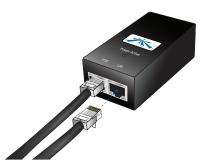
3. Connect the power cord to the power port on the *PoE Adapter*. Connect the other end of the power cord to a power outlet. The Power LED should light up on the airCam.
