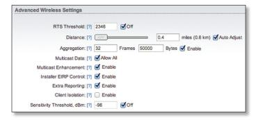
**Distance** To specify the distance value in miles (or kilometers), use the slider or manually enter the value. The signal strength and throughput fall off with range. Changing the distance value will change the ACK (Acknowledgement) timeout value accordingly.
