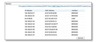
**IP Address** Displays the IP address assigned to a network device.
