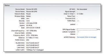
**airMAX Gateway** Displayed if your airMAX device is a CPE connected to an airMAX Gateway. You can click *Connected* (*Click to manage*) to remotely provision the airGateway.
