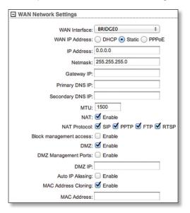
**IP Address** Specify the IP address of the device. This IP will be used for device management purposes.
