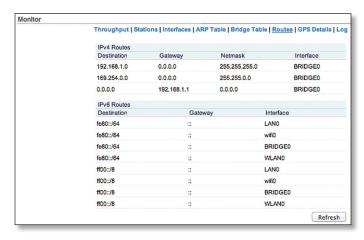
airOS examines the destination IP address of each data packet traveling through the system and chooses the appropriate interface to forward the packet to. The system choice depends on static routing rules, the entries that are registered in the system routing table. Static routes to specific hosts, networks, or the default gateway are set up automatically according to the IP configuration of all the airOS Configuration Interfaces.
