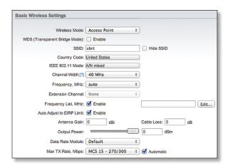
Access Point If you have a single device to act as an AP, configure it as Access Point mode. The device functions as an AP that connects multiple client devices. If you have multiple APs repeating signals where Ethernet connections are not readily available, then use AP-Repeater mode.
