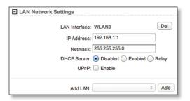
Enabled The device assigns IP addresses to client devices on the local network.
