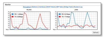
Throughput displays the current data traffic on the LAN and WLAN in both graphical and numerical form. The chart scale and throughput dimension (Bps, Kbps, Mbps) change dynamically depending on the mean throughput value. The statistics are updated automatically.
