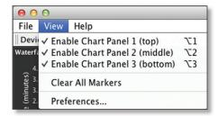
**Enable Chart Panel 1 (top)** Displays the Waterfall or Channel Usage chart in Chart Panel 1, depending on which option you have selected in *Preferences*. This time-based graph shows the aggregate energy collected or channel usage for each frequency since the start of the airView session.
