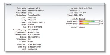
**SSID** Displays the wireless network name (SSID). The wireless network name depends upon the wireless mode selected:
