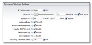
**RTS Threshold** (If airMAX is enabled, *RTS Threshold* is not required.) Determines the packet size of a transmission and, through the use of an AP, helps control traffic flow. The range is 0-2346 bytes. The default setting is the value 2346; this means that RTS is disabled.
