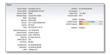
**Device Name** Displays the customizable name or identifier of the device. The Device Name (also known as host name) is displayed in registration screens and discovery tools.
