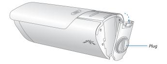
2. Connect the Ethernet cable to the Ethernet port.
