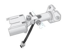
4. Unscrew the *Plug* on the back of the airCam.
