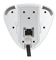
3. Insert the seal into the bottom of the camera and wrap the seal around the Ethernet cable. Reconnect the *Ethernet Door* to the airCam leaving the Ethernet cable fed through the seal at the bottom of the camera.
