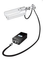
2. Connect an Ethernet cable from your LAN to the Ethernet port labeled **LAN** on the *PoE Adapter*.
