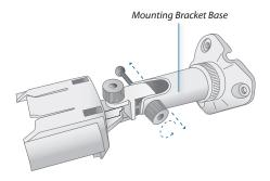
2. Insert an Ethernet cable through the *Mounting Bracket Base*.
