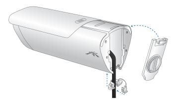
4. Insert the *Mounting Bracket* into the airCam until a click is heard to confirm a secure installation.
