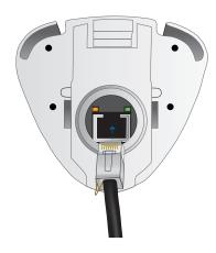
6. Insert the *Mounting Bracket* into the airCam until a click is heard to confirm a secure installation.
