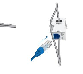
5. Connect the other end of the CAT5/6 cable from the mFi Current Sensor to an mFi RJ45 port on the mFi mPort.
