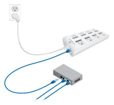
Wi-Fi The mPower PRO can connect to a wireless network once Wi-Fi settings have been configured using the Ethernet connection. For instructions, refer to the Accessing the Configuration Portal section.
