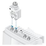
4. Attach the second Duplexer (not included) to the RX 1 and TX 1 ports, ensuring that the numbers on the adjacent sides of the Duplexers match. (The numbers on the Duplexer on the right should be in the reverse order of the numbers on the Duplexer on the left.)
