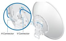
Attach the airFiber X radio to the antenna by aligning the four tabs on the back of the radio with the slots of the radio mount. Then slide the radio down to lock it into place.
