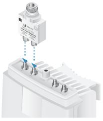
WARNING: Tighten the collars alternately, turning one collar a half turn, then the other collar a half turn, and so on, until both are fully tightened. Failure to do so may result in damage to the Duplexer. Reseat the Duplexer Shroud onto the AF-11FX radio and tighten the Captive Screw to secure the Duplexer Shroud.
