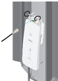
Connecting the GPS Antenna
