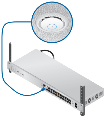
UniFi Switch Power Connection Diagram
